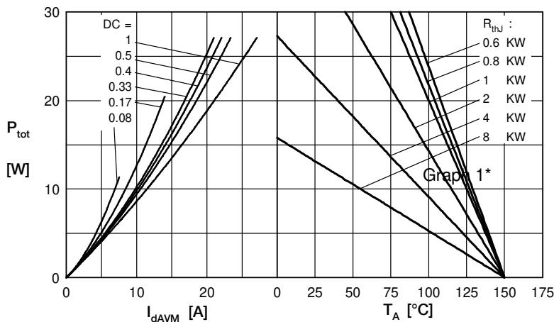
Fig. 4 Power dissipation vs. forward current
