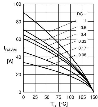
Fig. 5 Max. forward current vs.
